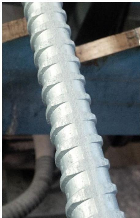
The assortment of the mill includes rolled sectioned hot-rolled screw threaded rebars intended for screw joints of structures in the mining and metallurgical, construction and engineering industries.
