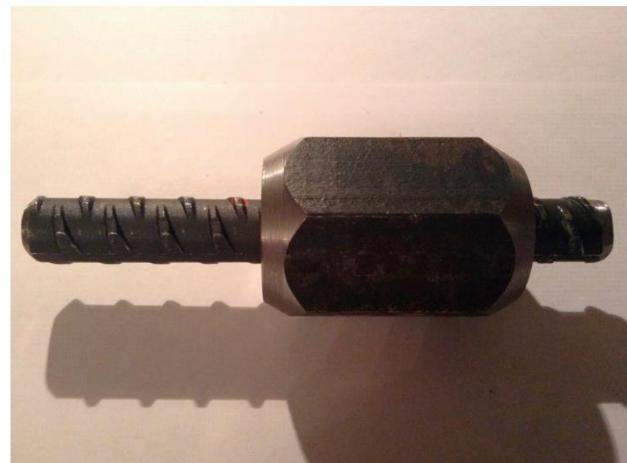
Connecting elements (couplings, locknuts, anchor nuts) are supplied by the Tula Metal Rolling Plant complete with rebars. They are made by cutting a standard hexagonal steel billet (GOST 2879-2006). It is possible to supply products made of a round steel billet, as well as by hot stamping and precision casting in compliance with the conditions for meeting the quality requirements of products obtained by metal cutting.
